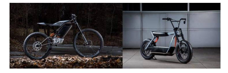
Just looking at the vehicles reveals a number of clues. The dirt bike is outfitted with large 3-4" off-road tires, an inverted front suspension fork, rear hydraulic reservoir suspension, a low-slung motor case that appears to perform double duty as a structural frame member, belt drive and a seat that says to me "you'll be standing on the pegs most of the time".
