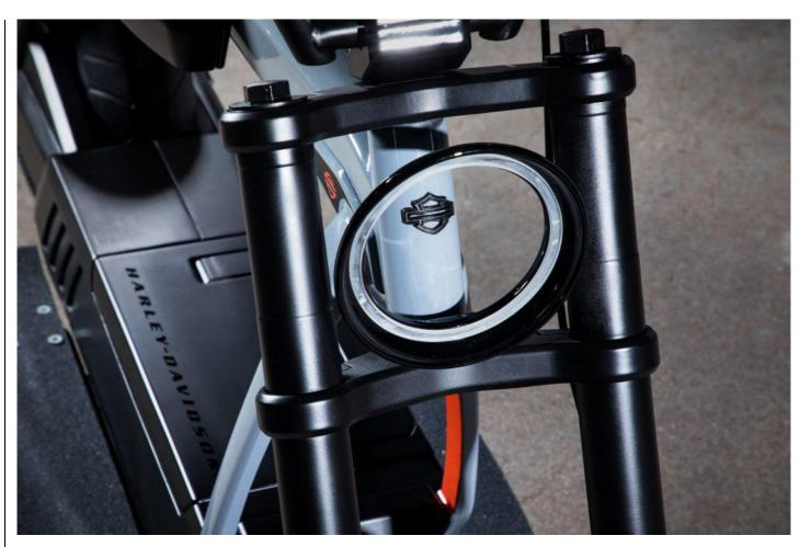
Lights include an impressive looking front LED halo headlight and a rear LED bar tail light. No turn signals are visible.
